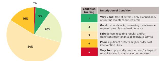
The Torrens Weir is an aging asset, originally constructed in 1881 with sluice gates added in 1929. Majority of its components are rated in a fair to poor condition and engineering inspections and recommendations have identified the need to undertake an options analysis (currently underway) to guide the future management of the asset as it approaches the end of its useful life.
